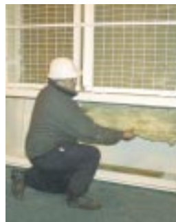
Filter material stores on top of booth, is easily accessible at floor level behind roll-up door.
