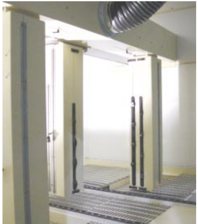
Booth interior features two fixed side-spray gun trees (left & right) and one traversing end-spray gun tree (center) in pressurized enclosures.
