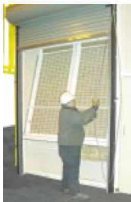
Filter material stores on top of booth, is easily accessible at floor level behind roll-up door.
